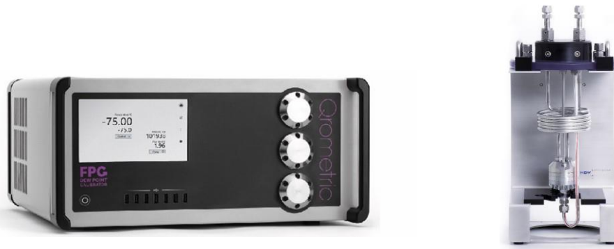
Figure 21: The Qrometric Frost Point Generator (FPG) and the PI/MBW SLX chilled mirror hygrometer calibrated at INRIM and used for its initial validation.
