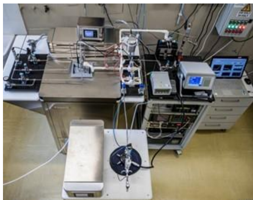
Figure 8: (Left) Calibration set-up of INRIM 03 Mk2 connected to a CMH and a CRDS analyser; (Right) Top view of the trace water generator manifold for 1-P and 2-P operation.
