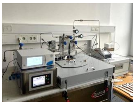
Figure 13: The new generator that withstands pressures up to 1 MPa (left panel) and the schematic diagram of the UL-FE/LMK low frost-point generator (right panel).
